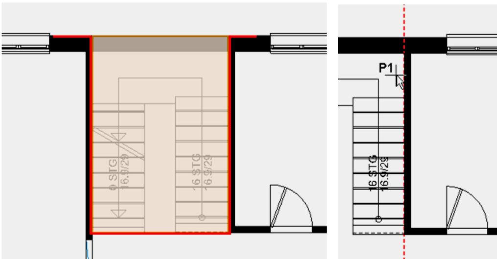
1. Apply a help line using the function PARALLEL STRAIGHTS with distance 0 to the staircase wall **P1**.
