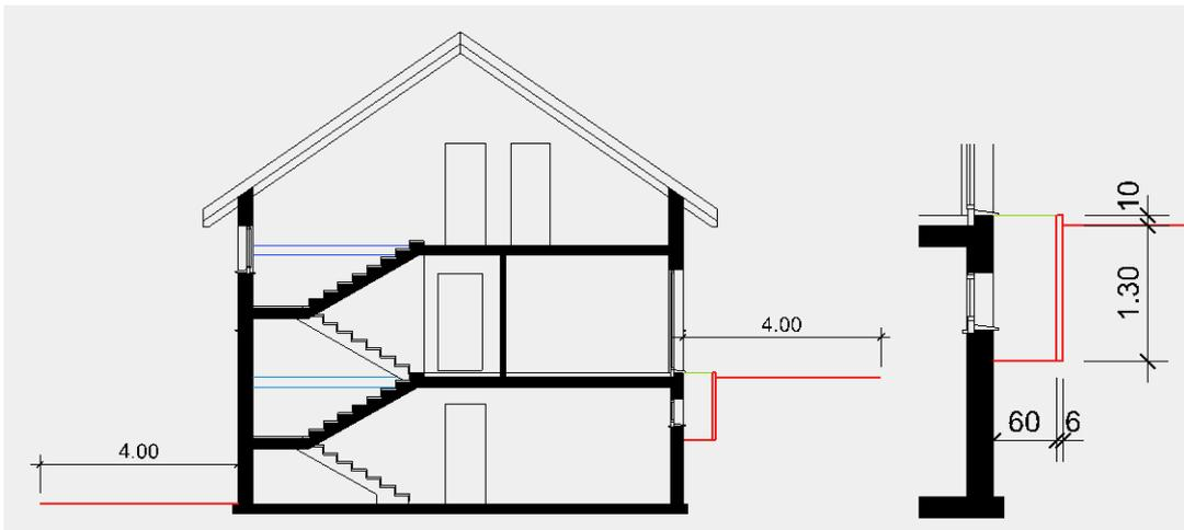
4. The floor finish is missing from the top floor and the basement.
