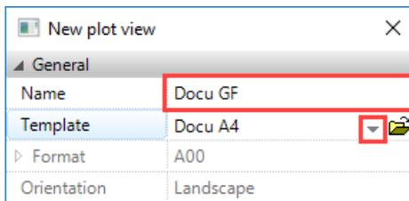
3. The new plot view appears with the layout template on screen. In the header line of views management, select the function INSERT VIEW and select the *GF* from the list.
