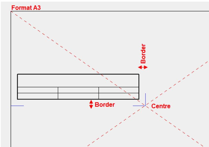
3. Add texts. To enable a text to be created vertically in the centre of a field, the text reference point must be set to *Centre left*.
