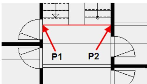
6. The last step projects into the door opening. The wall and the two doors must be moved.
