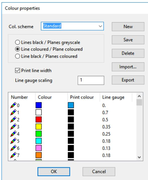
The same screen can also be accessed via the menu SETTINGS > COLOUR PROPERTIES. The print colour and line width of the individual pens can be modified.
