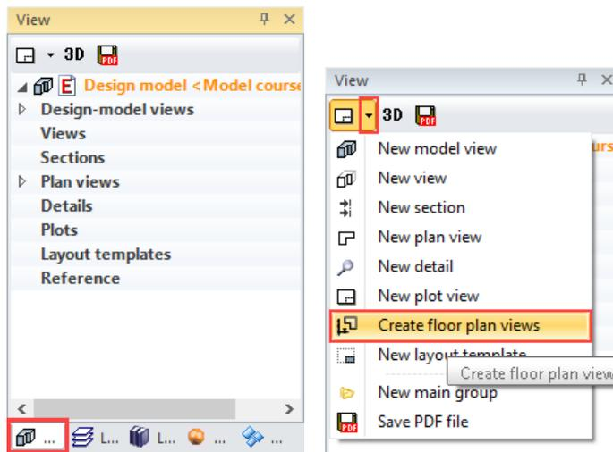
2. Create the floor plans using the function GENERATE FLOOR PLAN VIEWS.
