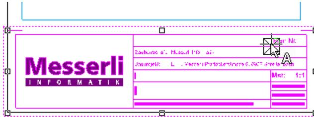
6. Select the COPY function and place the reference point at the bottom right.
