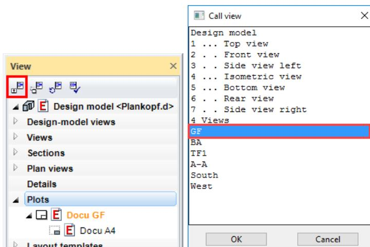
4. Insert the ground floor into the plot.
