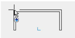
As soon as the library part is attached to the cursor, the properties bar appears. To enable the light shaft to be better placed, you must move the reference point.
