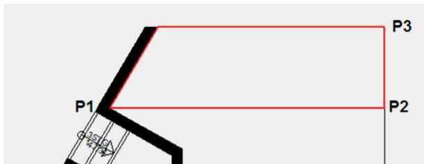
3. You must now specify a height for 3 points of the plane. Click on the corner at **P1**, in the input line enter the height **160** and confirm the value.
